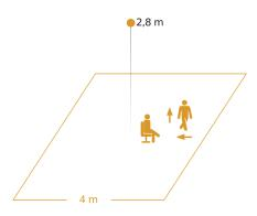
Possible mounting height: 2,50 m - 4,00 m Orange: presence, tangential and radial
